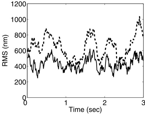
FIG. 3.—Wavefront aberration averaged over the 6.5 m pupil for a representative sample of data. The dashed line shows the total for the reconstructed modes in Zernike orders 2–6 in the stellar wavefront. The solid line shows the residual after subtraction of the average RLGS wavefront.
