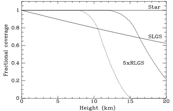
FIG. 7.—Fractional intersection vs. height of the area covered by light from an axial star and three LGS beacon arrangements: a single axial sodium laser guide star (SLGS) at 95 km range and pentagonal constellations of Rayleigh laser guide stars (RLGSs). We show the cases of a 6.5 m aperture with the RLGs on a  $60''$  radius at 24 km range (*dotted line*) and an 8.0 m aperture with RLGs on a  $43''$  radius at 30 km range (*dashed line*).
